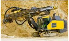
When equipped with the standard feed option, the FlexiROC D65 is capable of handling an even wider range of jobs with ease, including drilling de-watering holes.
